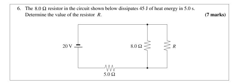
$P_{8.0\Omega} = 45/5.0$   $P_{8.0\Omega} = 9.0 W \quad \leftarrow 1 \text{ mark}$   $9.0 = (I_{8.0\Omega})^2 \cdot 8.0$   $I_{8.0\Omega} = 1.06 A \quad \leftarrow 1 \text{ mark}$   $V_R = V_{8.0\Omega} = 1.06 \cdot 8.0 = 8.48 V \quad \leftarrow 1 \text{ mark}$   $I_R = I_{circuit} - I_{8.0\Omega}$   $I_R = (20 - 8.48)/(5.0) - 1.06$   $= 1.24 A \quad \leftarrow 2 \text{ marks}$  R = 8.48/1.24  $= 6.8 \Omega \quad \leftarrow 2 \text{ marks}$
