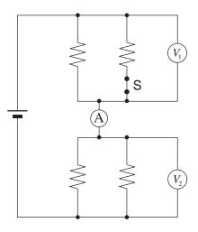
If the switch is then opened, what effects will be observed in the readings of the three meters? (All resistors have the same value.)
