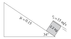
a) Determine the magnitude of the force due to friction which acts on the paint can as it slides up the incline. (2 marks)
