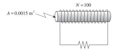
If the magnetic field in the iron core changes from 3.0 T towards the left to 1.0 T towards the right, how much charge flows in the circuit?
