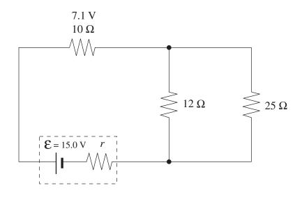
a) What is the power dissipated by the 25  $\Omega$  resistor?
