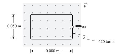
The magnetic field strength is increased over a 0.20 s interval, inducing an average emf of 1.8 V in the coil. What is the final magnetic field strength? (7 marks)
