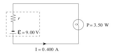
a) If a current of 0.400 A leaves the battery, what is the internal resistance, *r*, of the battery? (5 marks)
