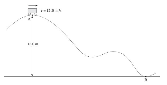
What is the speed of the roller coaster at point B at the bottom of the hill if 8 500 J of energy is transformed to heat during the journey? (7 marks)
