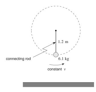
a) Draw and label a free body diagram for the object at the bottom of the circular path. (2 marks)
