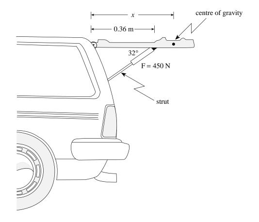
a) Draw and label a free body diagram showing the forces acting on the door. (2 marks)
