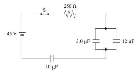
What is the charge on the  $3.0 \,\mu\text{F}$  capacitor?
