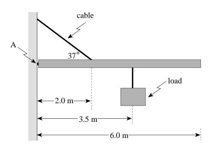
If the maximum tension the cable can withstand is  $2.4 \times 10^3$  N, what is the maximum mass of the load? (7 marks)
