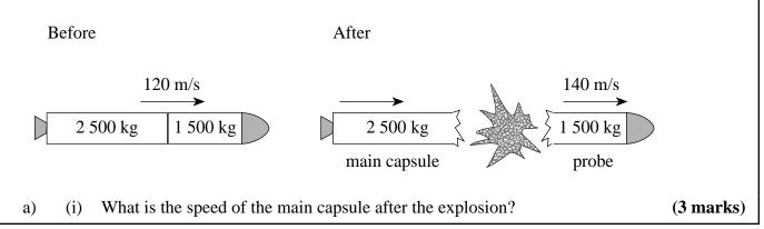
$$\begin{array}{l} m_{1}v_{1} + m_{2}v_{2} = m_{1}v_{1}' + m_{2}v_{2}' \\ (m_{1} + m_{2})v = m_{1}v_{1}' + m_{2}v_{2}' \\ (4\ 000)(120) = (1\ 500)(140) + (2\ 500)v_{2}' \quad \leftarrow 1 \text{ mark} \\ 270\ 000 = 2\ 500v_{2}' \\ v_{2}' = 108\ \text{m/s} \end{array} \right\} \leftarrow 1 \text{ mark} \\ \therefore \text{ speed} = 1.1 \times 10^{2} \text{ m/s}$$
