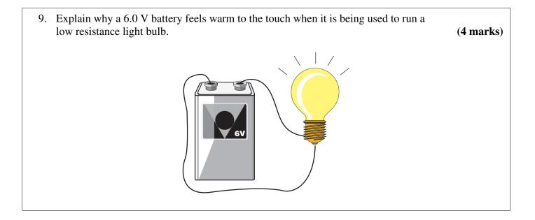
Low resistance light bulb will result in a high current through the battery (1 mark). This high current is passing through the battery's internal resistance (1 mark), resulting in the dissipation of an appreciable amount of heat (2 marks).
