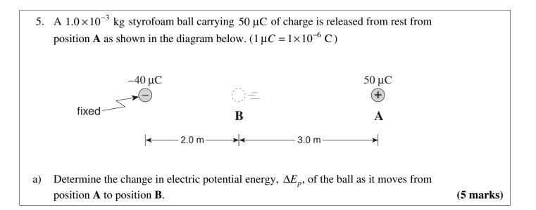
$$\Delta E_{p} = k \frac{Q_{1}Q_{2}}{r} - k \frac{Q_{1}Q_{2}}{r_{0}} \qquad \leftarrow 1 \text{ mark}$$
