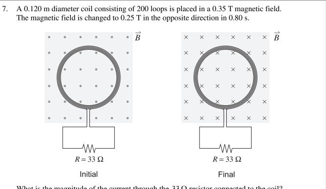
What is the magnitude of the current through the  $33 \Omega$  resistor connected to the coil? (Ignore the resistance of the coil.) (7 marks)
