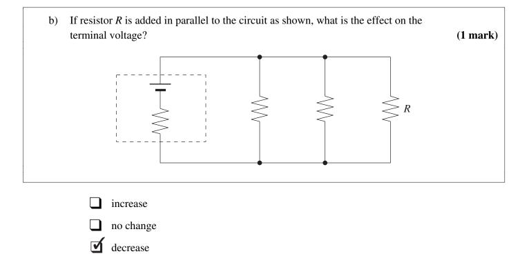
Additional *R* in parallel results in an overall lower *R*, thus an increase in current. (2 marks) As a consequence, a greater voltage drop *Ir* occurs across the internal resistance resulting in a smaller terminal voltage. (2 marks)
