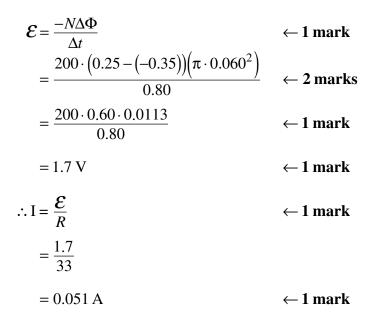
8. A conducting loop is pulled at various speeds through a region of constant magnetic field strength.
