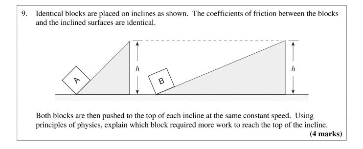
Work = Force  $\times$  Distance (1 mark). To move either block up the ramp, friction must be overcome. In the case of block B, the force of friction is greater (1 mark) and the distance is longer (1 mark). Therefore more work is done moving block B to the top of the ramp (1 mark).
