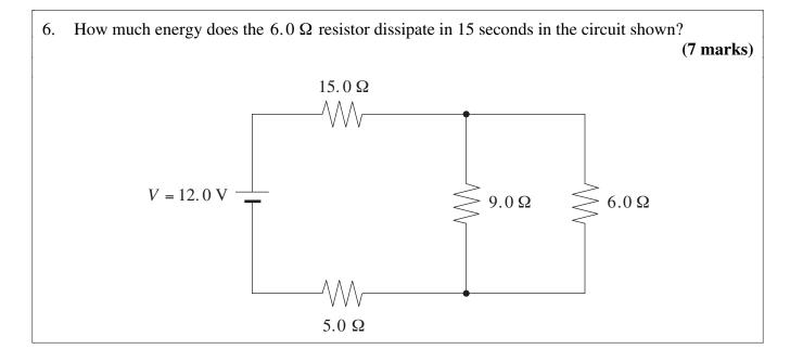
$\frac{1}{R_p} = \frac{1}{9.0} + \frac{1}{6.0}$  $R_p = 3.6$ ←1 mark  $R_T = R_{15} + R_p + R_5$ = 15.0 + 3.6 + 5.0= 23.6 Ω ← 1 mark  $I_T = \frac{V_T}{R_T} = \frac{12.0}{23.6}$ = 0.508 A ← 1 mark  $V_p = V_T - V_{15} - V_5$  $= 12.0 - 0.51 \times 15.0 - 0.51 \times 5.0$ = 1.83 V ← 2 marks  $I_6 = \frac{V_p}{R_6} = \frac{1.83}{6.0}$ = 0.305 A←1 mark E = VIt $= 1.83 \times 0.305 \times 15$ = 8.4 J←1 mark
