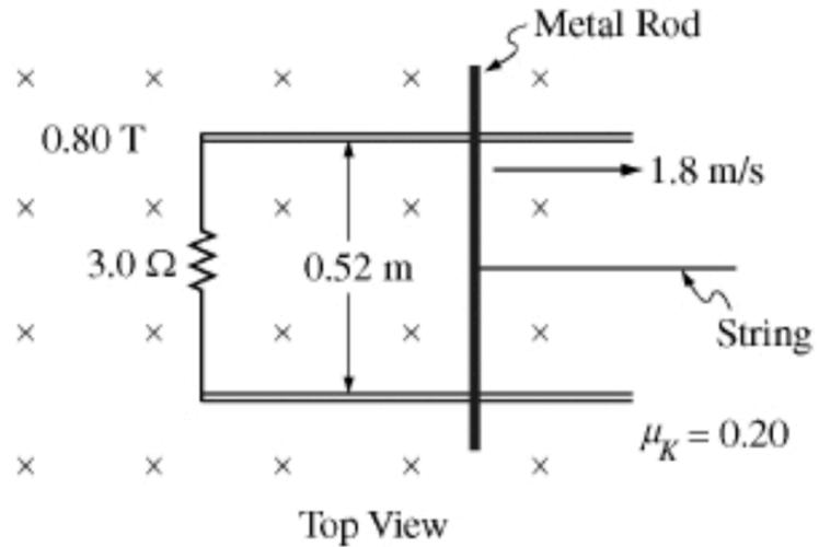
There is a magnetic field of  $0.80\ \text{T}$  perpendicular to the plane of the tabletop. A string pulls the metal rod to the right with a constant speed of  $1.8\ \text{m/s}$ .
