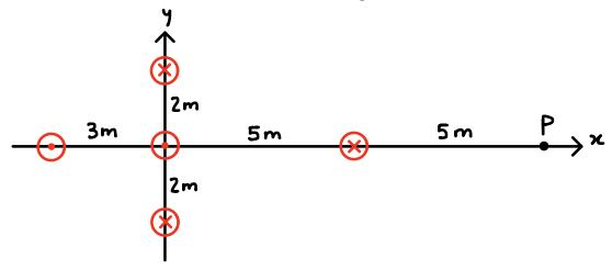
The magnetic field <u>outside</u> a solenoid is zero. As *P* is outside all five solenoids, the magnetic field at *P* is zero.
