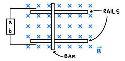
By the right hand rule, for the force on the bar to be to the right, current in the bar must be flowing down. This would mean *a* is positive.
