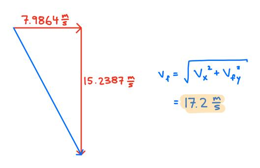
A launcher angled at 30° as shown is used to fire a ball towards a student 8.0 m away. At what speed must the ball be fired in order to hit the student?
