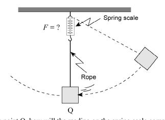
As the mass passes point Q, how will the reading on the spring scale compare to the previous value of 14 N? Using principles of physics, explain your answer.
