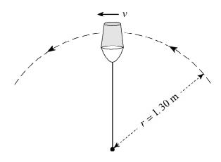
What is the minimum speed, v, at the top of the circle if the water is not to spill from the pail?
