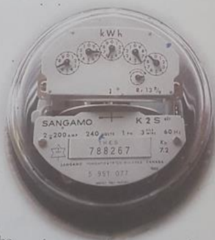
Figure 9.17 The electricity meter in your home may be similar to this one. The middle disk turns, showing the rate at which electrical energy is being used within the home.
