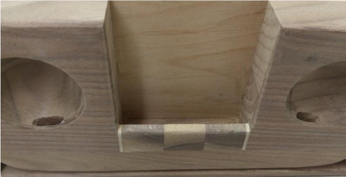
14. Angle the table saw blade 13 degrees and cut the bottom so that the woodtuth leans back.
