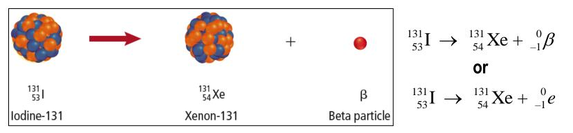
lodine-131 releases a beta particle and becomes xenon-131. A neutron has turned into a proton and the released electron. See page 296
