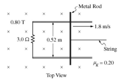
There is a magnetic field of 0.80 T perpendicular to the plane of the tabletop. A string pulls the metal rod to the right with a constant speed of 1.8 m/s.
