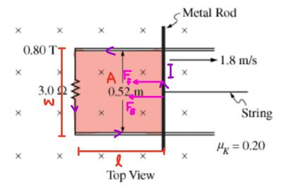
There is a magnetic field of 0.80 T perpendicular to the plane of the tabletop. A string pulls the metal rod to the right with a constant speed of 1.8 m/s.
