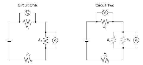
How have the values of  $V_1$  and  $V_2$  in circuit two changed compared to those in circuit one?
