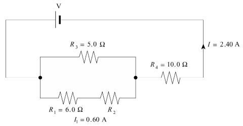
b) Find the potential difference of the power supply, V.
